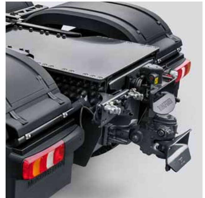
Heavy-duty trailer coupling. The Rockinger 56 E heavy-duty trailer coupling is designed for loads up to 250 t. It can be fitted in two different positions on the heavy-duty cross member.
