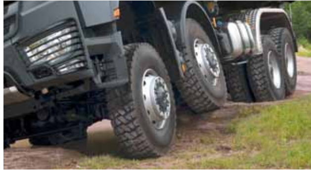
Axle load compensation The axle load compensation between the front axles prevents overloading damage on 8x6 and 8x8 vehicles.
