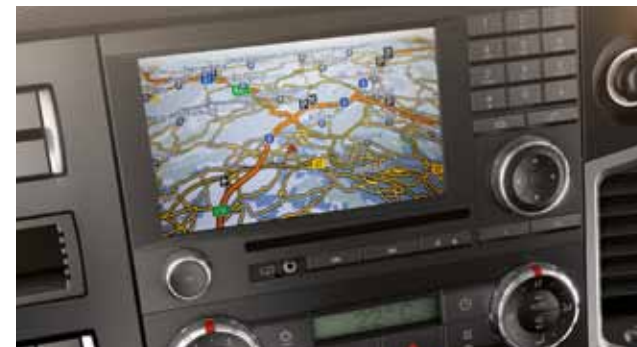
Bluetooth® Radio Navigation System 1 . Equipped with a 17.4 cm colour display as well as Bluetooth® and convenience features, the system leaves nothing to be desired when it comes to support for the driver and entertainment.
