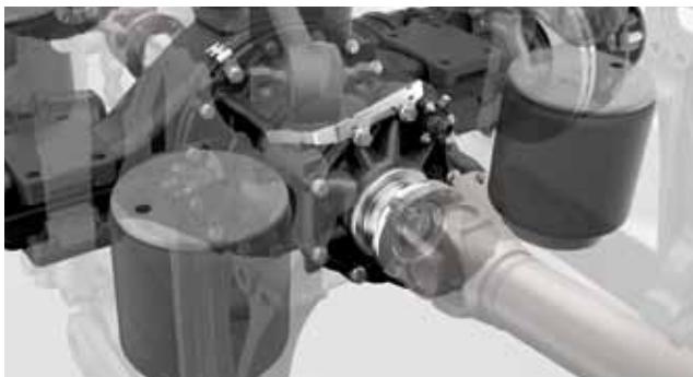
Rear axle, crown wheel 440, hypoid, 13.0 t. The rear axle is a weight-optimised sheet-steel formed axle with a 440 mm ring gear. It is fitted to air-suspended 3-axle vehicles up to a gross train weight of 80 t and from 2200 Nm.
