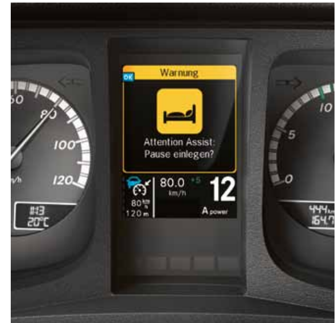
Attention Assist 7) . The system can recognise increasing tiredness and recommend the driver takes a break 2) 7) 8) .
