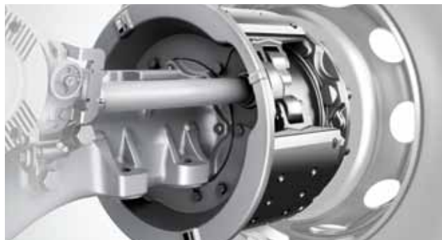
Full brake power at all times. Highly robust for maximum safety: depending on the intended application, drum brakes, a combination of disc and drum brakes or disc brakes ensure short stopping distances for the Arocs.
