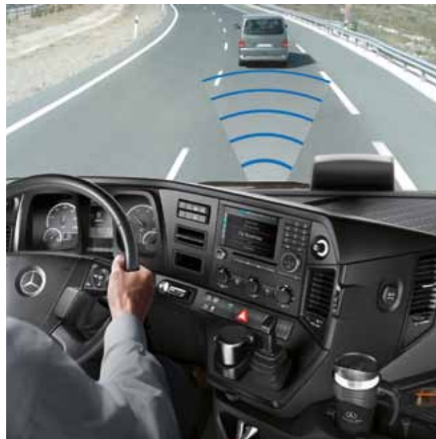
Proximity Control Assist 1) 2) 6) . The safety system with stop-and-go function is on hand to support the driver in stressful situations and can reduce the risk of rear-end collisions.
