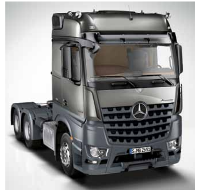
BigSpace L-cab. With standing headroom of 1.99 m between the seats, the cab with a level floor and measuring 2500 mm in width offers unusually generous freedom of movement and comfortable through-access to the co-driver's side.
